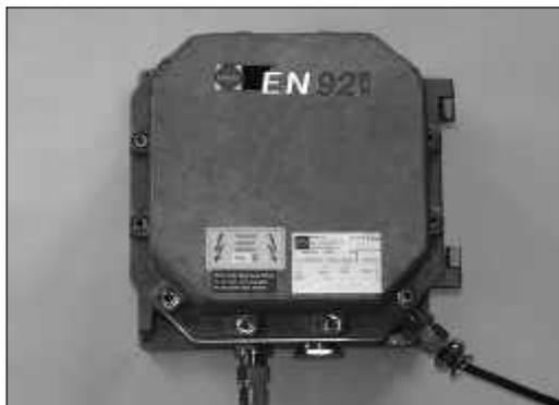
Power pack **EN 92 Ex** is suitable for direct use in areas with potentially explosive atmospheres (zones 1 or 2). The units comply with the European ATEX directives. All high-voltage components are accommodated in a flameproof housing.
